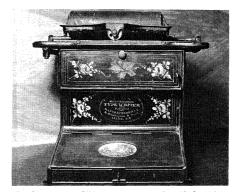
The Sholes and Glidden typewriter of c. 1873, which. with refinements, became the Remington Model 1 By courtesy of Remington Rand Office Machines Divis
